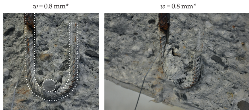
Figure 3.20 Saw-cut performed after test in specimen SB14 with deformed hooks disposed parallel to cracks with long bar (dashed line for initial position and geometry of the detail)
