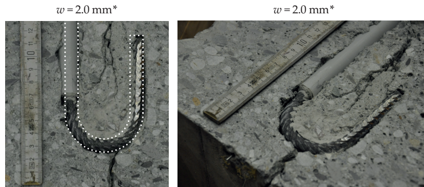
Figure 3.21 Saw-cut performed after test in specimen SB13 with deformed hooks disposed perpendicularly to cracks (dashed line for initial position and geometry of the detail)
