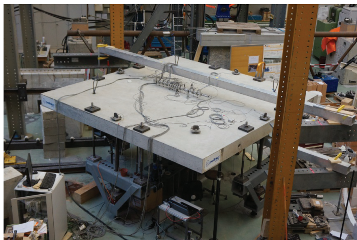
Figure 1.2 Full-scale punching test on an isolated specimen, supported on a column in the center and loaded at 8 points close to the perimeter [Ein16a]
