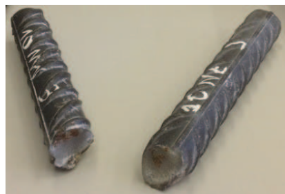
Figure 5.12: Failed rebars due to fatigue
