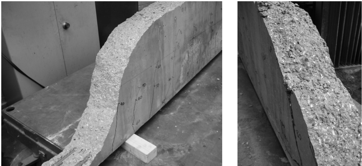
Figure 6.28: Crack surfaces: Left - Limestone aggregate beam; Right - Gravel aggregate beam
