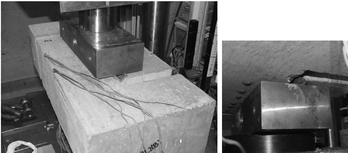
Figure 4.4: Pre-cracking of push-off specimens ( Left – Top view; Right – Bottom view )
