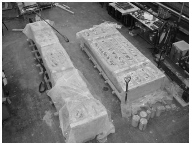
Figure 6.6: Left - Moulds for beams AL4 to AL0 (left to right); Right - Casting of gravel beams
