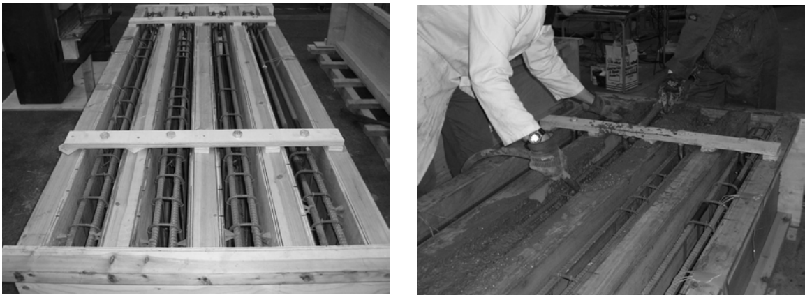
Figure 6.6: Left - Moulds for beams AL4 to AL0 (left to right); Right - Casting of gravel beams
