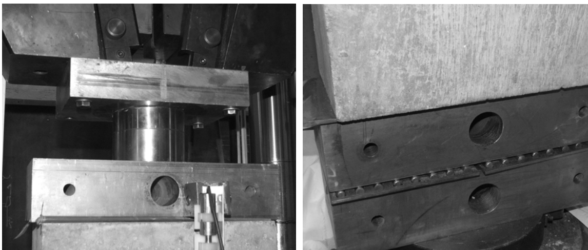
Figure 4.3: Left – Top loading plates and spherical seating; Right – Release of horizontal displacements at the bottom support by using mini-rollers
