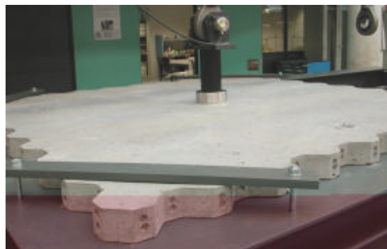
Figure 13. Punching test on BHP slabs, 70 mm thickness.
