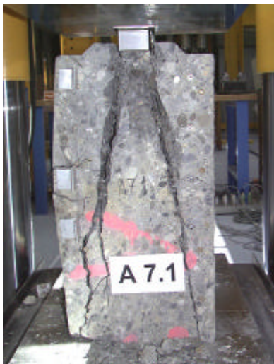
Figure 14. Study on the joints of tunnel segments (compression and punching of transverse and longitudinal joints).
